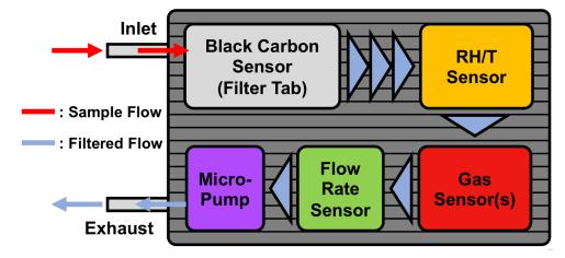
The ObservAir's micropump draws air through the fibrous aerosol filter. As particulate matter accumulates on the filter, the **aerosol absorption photometer** measures the rate of 880 nm light attenuation and calculates **black carbon** concentrations. Downstream, a **relative humidty and temperature (RH/T)** sensor monitors environmental conditions and **electrochemical cells** measure up to **two gaseous pollutants** simultaneously.
